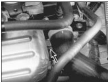
6.9 Location (arrowed) of coolant temperature gauge sender
