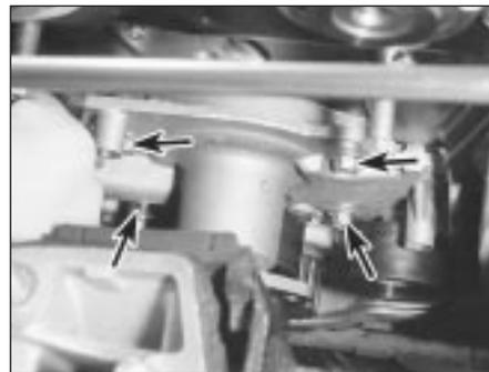
**8.9 Unscrew bolts (arrowed) . . .**
