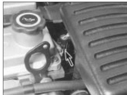
6.15 Location (arrowed) of coolant temperature sensor
